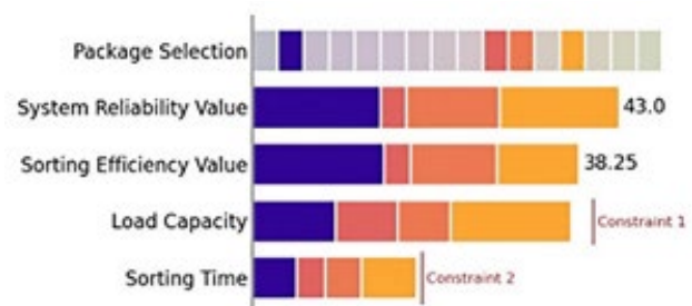
Fig 12. Multi-objective consolidated sorting based on predicted reliability and efficiency values, under the constraints of truck loads and sorting time.
